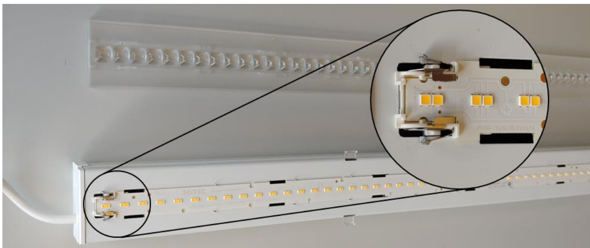
Figure 6: Zhaga Book 21 connector designed into the Repro-light exchangeability demonstrator
